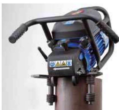
Edge machining on vertical pipes
