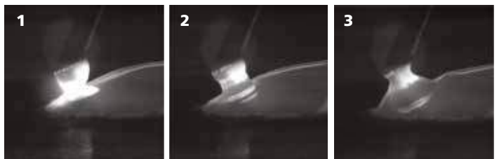
IAC - Vertical downward welding of a root pass in a district heating pipe. Welding speed is significantly increased compared to traditional upward welding..
